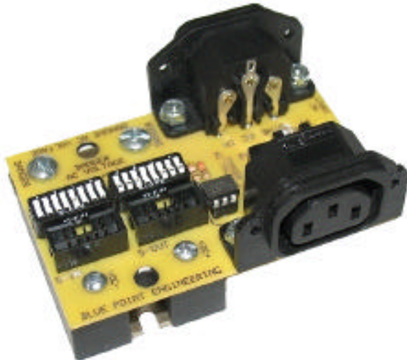
Solid State AC Power Switch (110-AC @ 5 Amp Loads) (1-Ch RX Board )
