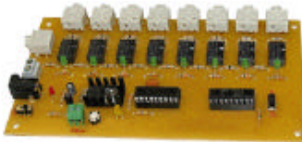
8-Ch Audio Sequence Switch Board (1-Ch Receiver)
