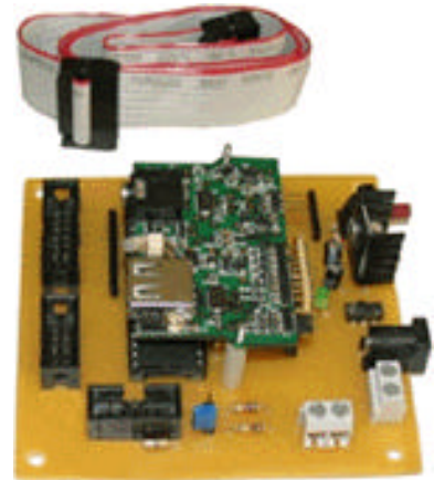
8-Ch Selectable MP3 Audio Playback (8-Ch Receiver)
