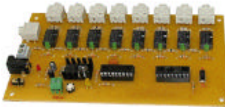
8-Ch Audio Sequence Switch Board (1-Ch Receiver)
