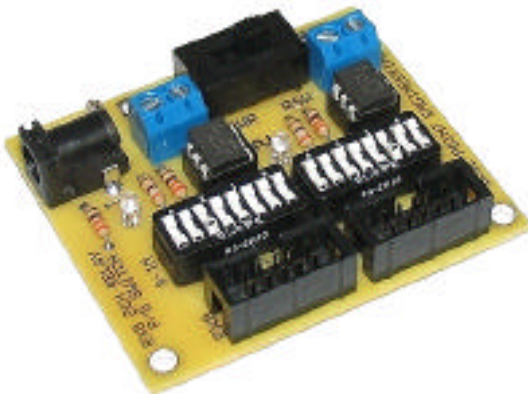
1-Ch SS Relay Power Switch 1-Ch SS Relay Switch (1-12VDC @ 2 Amps)
