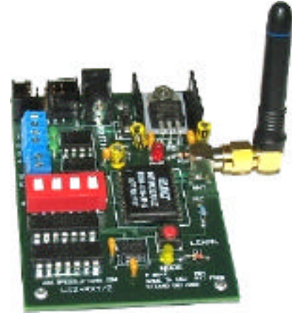
4-Ch Receiver (RX) 4-Ch Ribbon Connector 4-Ch on-board output blocks
