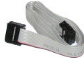
Connection Cable to Application Boards (RX - Application)
