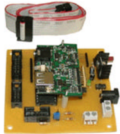
8-Ch Selectable MP3 Audio Playback (8-Ch Receiver)
