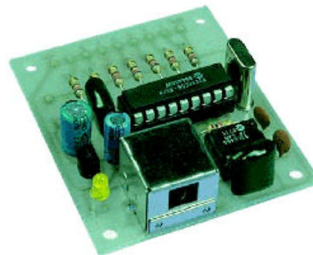
Board Size: 2-1/4" L x 1-3/4" W Power Requirements: 9Volt dc @ 0.5 Amp
