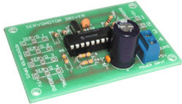
Board Size: 2-7/8" L x 2" W x 1" H Power Requirements: 5Voldtc @ 2 Amp
