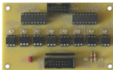
4-Ch Servo Controller to RX8M/Receiver Interface Board
