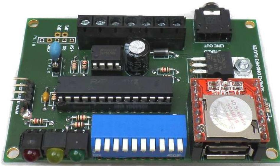
Compact DMX512 controlled MP3 player based on the 4D Systems' SOMO-II module. Control the playback of up to 255 MP3 format tracks using either uSD or USB pen-drive media.
